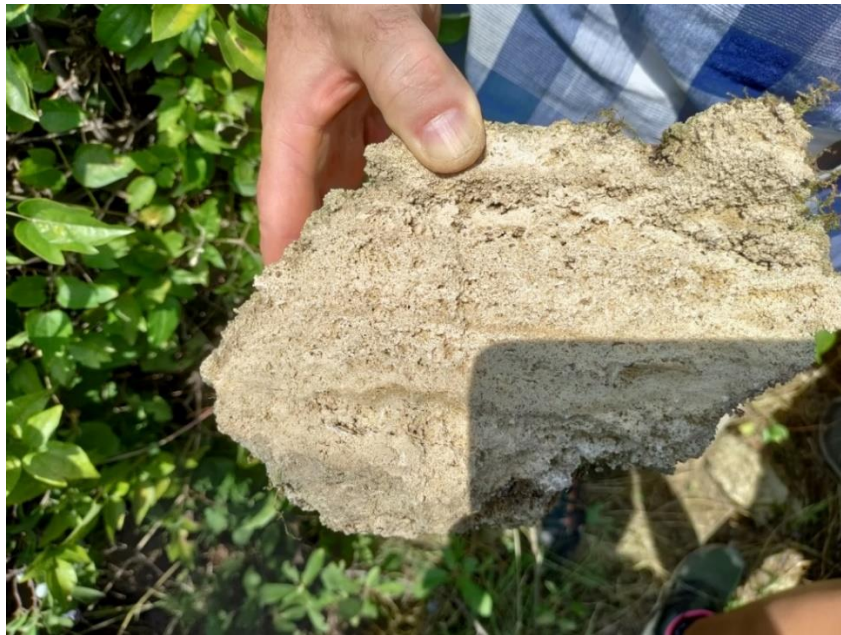
Photo 6. shows the porous structure of the Pleistocene freshwater limestone (Photo taken by K Pesztranszki).
